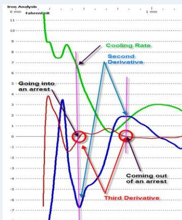
So in thermal analysis we look for not just how much the cooling rate changes, but how fast the cooling rate changes. Since the cooling rate is  $1/1^{\text{st}}$  derivative, the rate of change or slope of the cooling curve (Green) is the second derivative (Blue). The highest rates of change will be marked by the  $3^{\text{rd}}$  derivative (Red) crossing zero.
