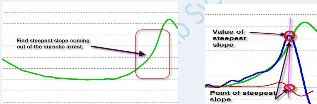
That value is the steepest slope of the cooling rate, or the maximum 2<sup>nd</sup> derivative value (blue) which the computer finds when the 3<sup>rd</sup> derivative (red) crosses zero.
