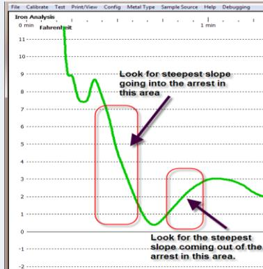
below 0.2 degrees C. This limitation could not tell the user how much over inoculated the metal was and therefore how much to cut back on the inoculation.
