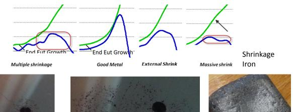
Looking at the graph to the right, the "dips" in the blue curve (red boxes) indicate endothermic or heat absorbing events in the sample. What is happening at these moments is the formation of an interior surface – something we associate with shrinkage.<sup>ii</sup>
