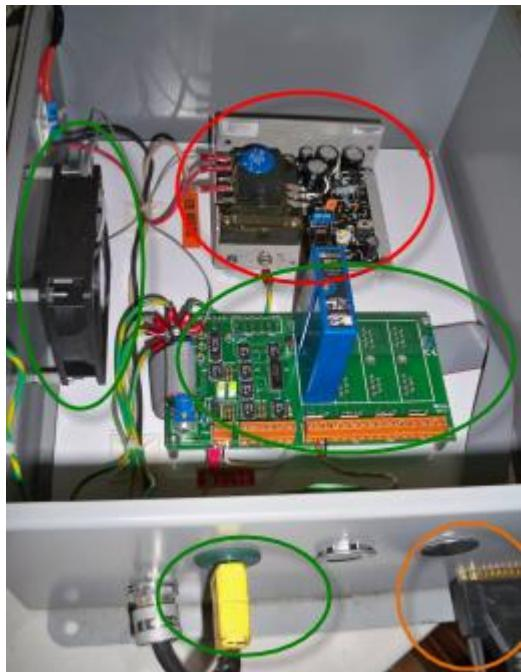
The red circled is a steady state transformer that keeps the voltage to the converter steady at 5.0 VDC with less than 0.01 VAC. This is the 1.5 amp version with enough power for 4 inputs. Life expectancy is > 10 years. Occasionally the output voltage may need tweaking.
