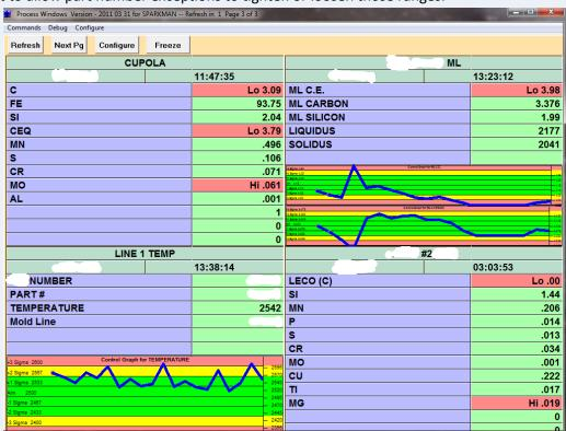
Dates, process names and part numbers have been erased in the above example to preserve the identity of the foundry. But here you can see spectrometer, LECO® and MeltLab® data combined, flagged if high
