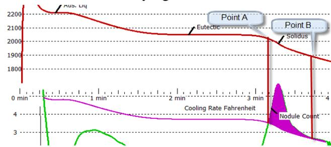
proportional to the energy absorbed by the strange feature. Ratioed against the rest of the curve, the area reaches a maximum of 10 to 12 percent of the total energy of solidification. The answer we came up with was that this is stress in the grain boundary. As the area decreases the stress is being relieved either through shrinkage or suck-in.
