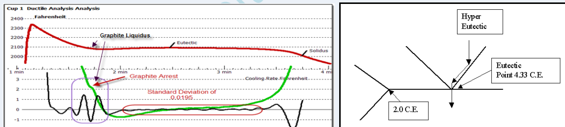
Fig 1. A final hyper-eutectic ductile iron curve showing a tiny near invisible graphitic liquidus arrest.
