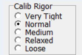
Once the necessary rigor has been met, the calibration window for that input turns green and the correction is locked. You can then move to the next input if you need to.
